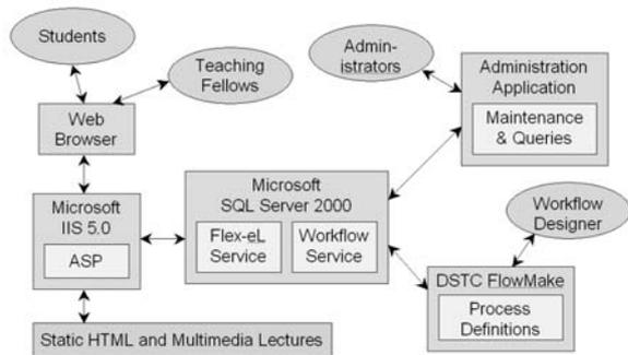
**Figure 1. Flex-eL Technology Architecture**
