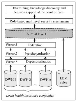
Figure 5. Phases of data warehouse consolidation
