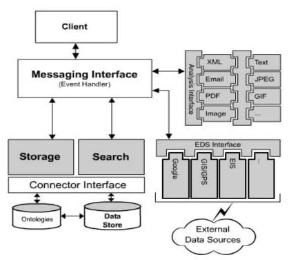
Figure 1. Architecture for 'SemanticLIFE' Framework
